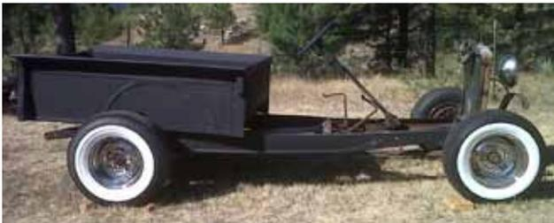
1932 Ford pickup rolling chassis includes: pickup bed; four 15" chrome reverse wheels; original 'K' member and cross members; front fender braces; radiator; headlight bar; and steering box and column with original key in column lock. The torque tube and rear end were chromed in the 1960's
